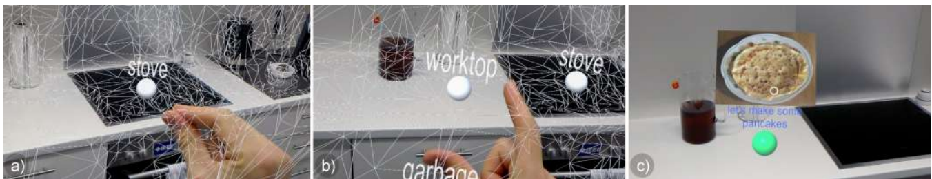
Figure 1: Locations for in-situ instructions are positioned in the room via gaze pointer (i.e., the current location to be positioned is following the current gaze direction) and AirTap gesture (a). This way, virtual locations can be attached to their real-world counterpart (b) to present instructions at their corresponding position (c).
